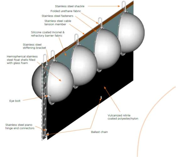
Figure 1. Desmi illustration of Desmi Pyroboom construction features
