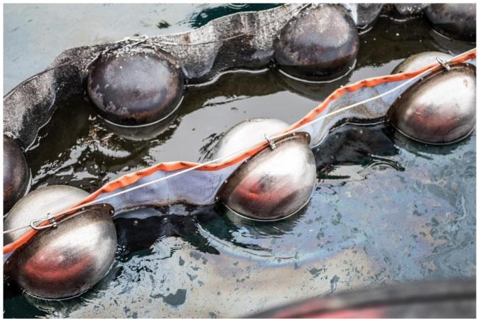
Figure 2. Picture of Desmi fireboms after termination of both burns
